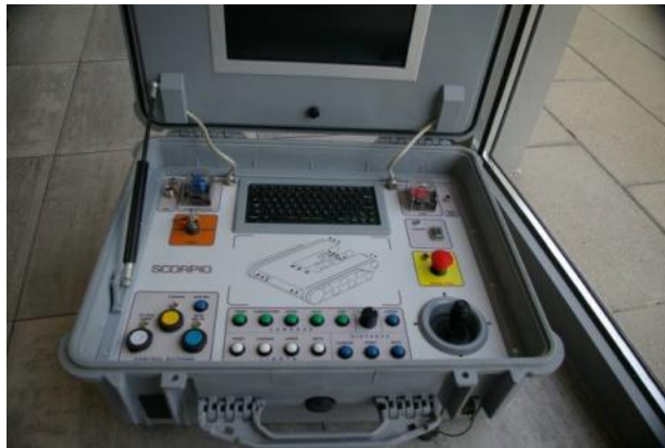
Fig. 2. Portable briefcase used for remote control of the robot SCORPIO.
